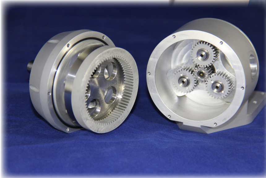
Disassembled All-Alloy Planetary Gear Box
