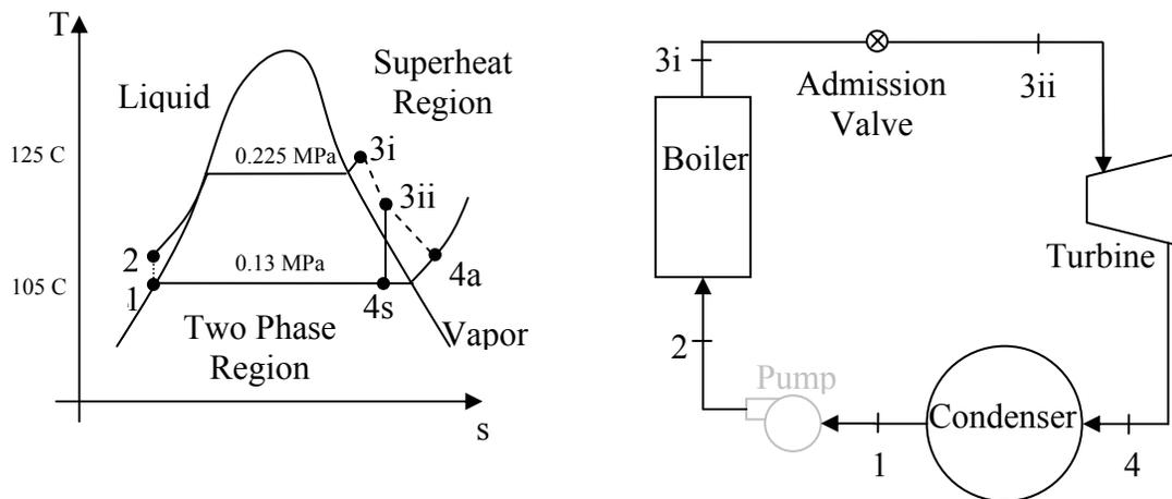
Figure 7: T-s Cycle Diagram, Idealized Straight-Line Expansion
