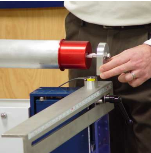
Insert Cantilever Load Block on red end.
