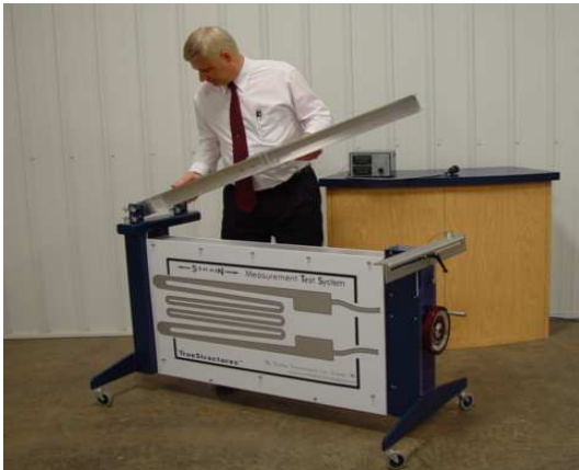
Position I-Beam Assembly Into Frame
