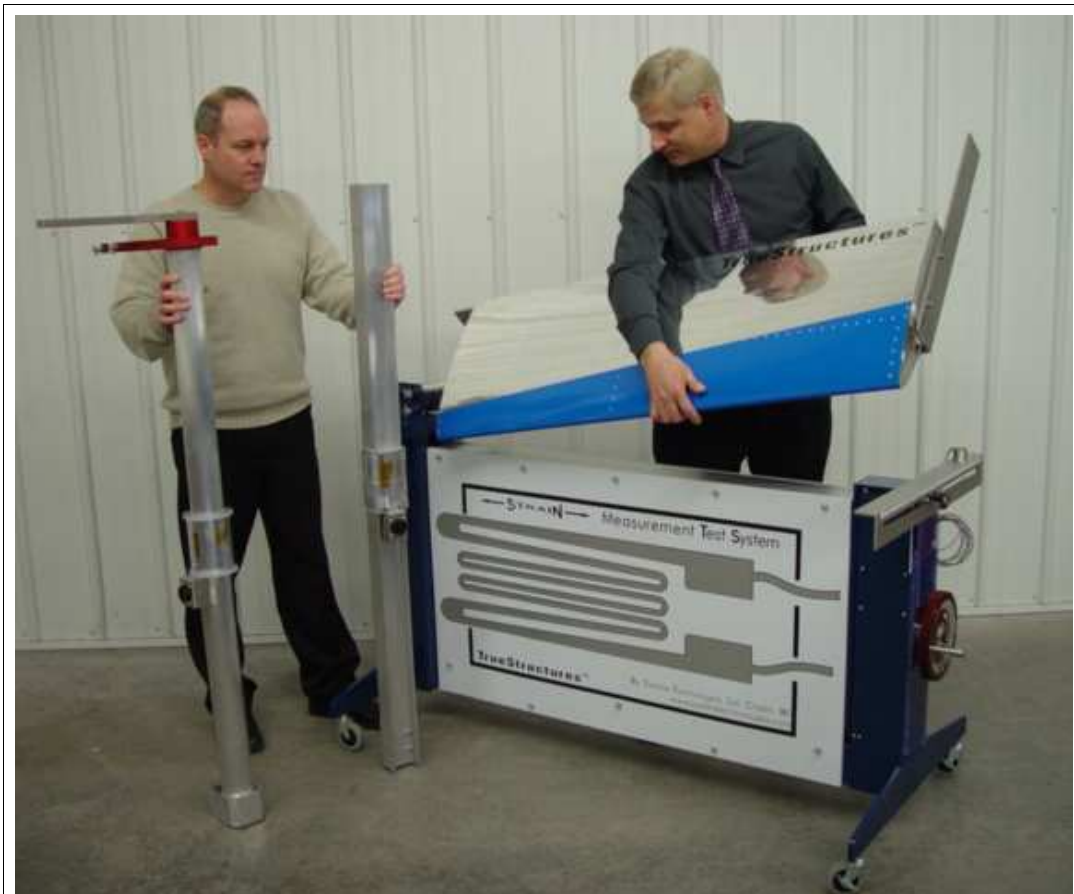
TrueStructures™ Strain Analysis System shown with I-Beam, Torsion Tube and Airfoil Test Sections.
