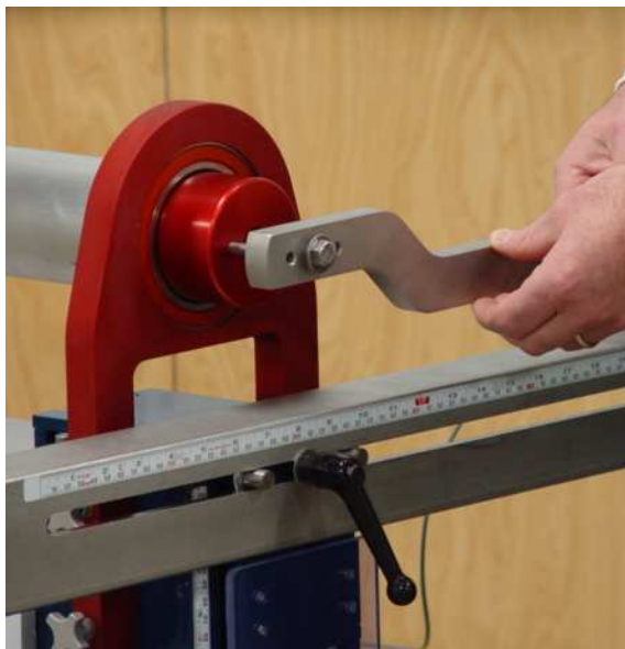
Position guide pins and slide on Torque Arm
