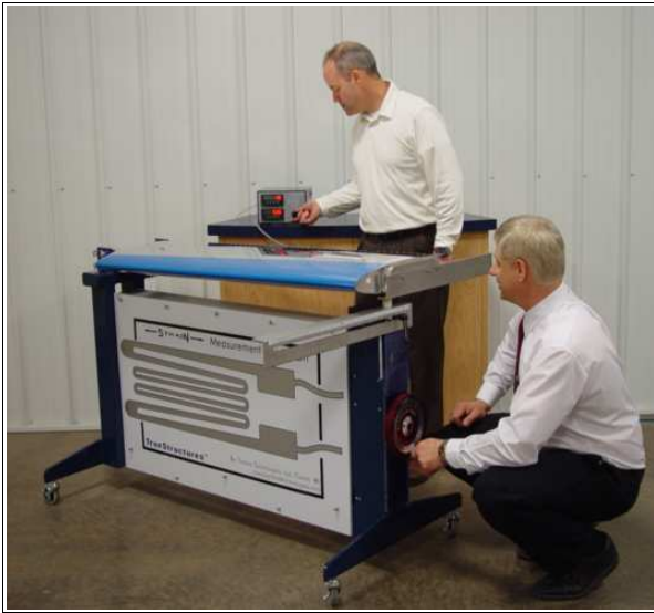
Taking readings from front wing spar loading.
