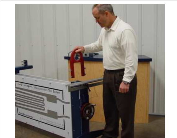
Position Yoke on Crank End (note correct face out as marked)
