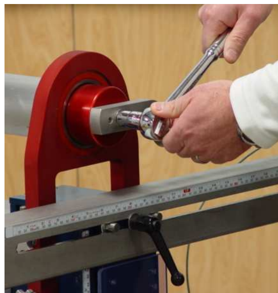
Tighten Torque Arm Bolt securely with socket wrench.
