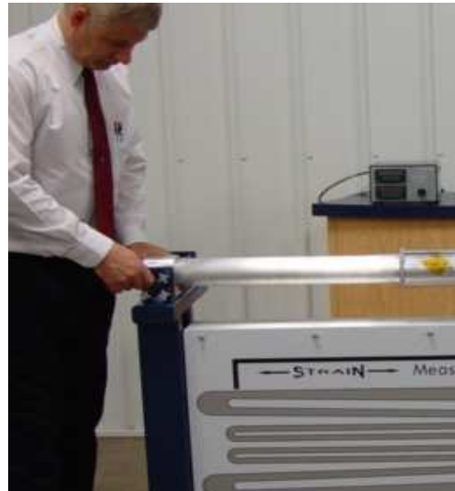
Tighten block end knobs fully. Then tighten red yoke knobs securely.
