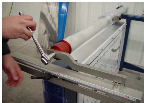
Tighten Arm with Socket Wrench, then position Load Cell.
