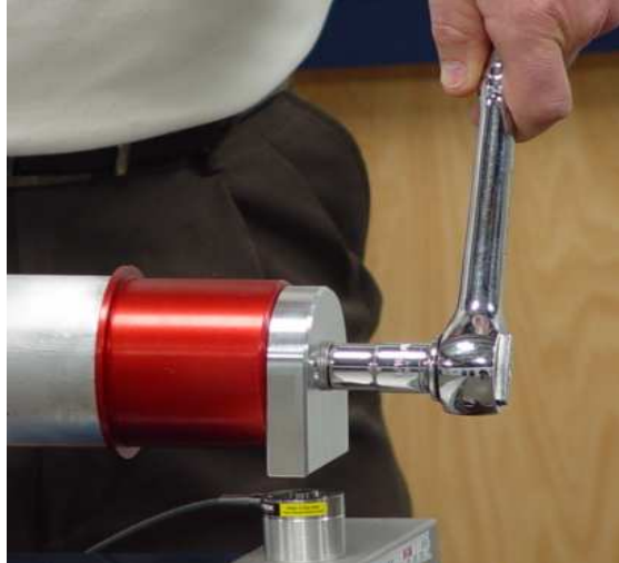
Tighten Load Block with socket wrench.
