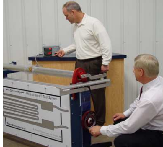
Crank in load and take readings on each channel (Steps 3, 4, 5) .
