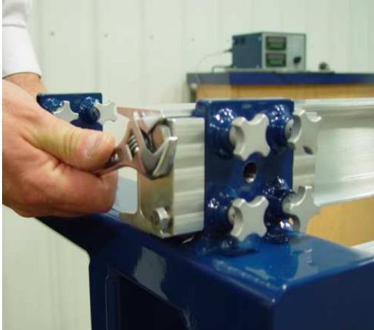
Tighten end bolts for sag-free connection.
