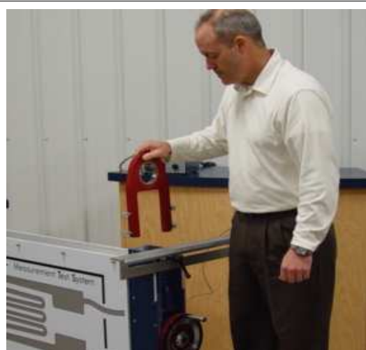
Loosen capture knobs, remove yoke.
