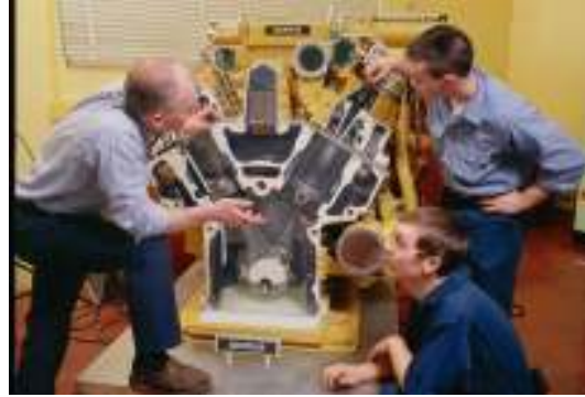
© MMA retains all creative rights Figure 4: Diesel Lab Cutaway Caterpillar Engine
