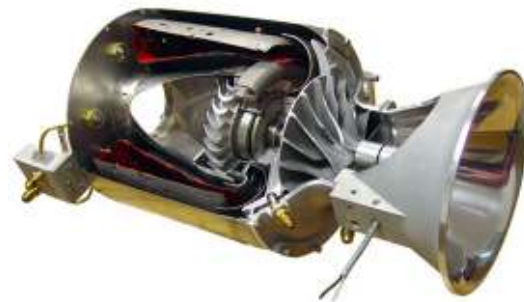
Figure 5: SR30 Cutaway view of Micro-turbine (Illustration from www.turbinettechnologies.com )
