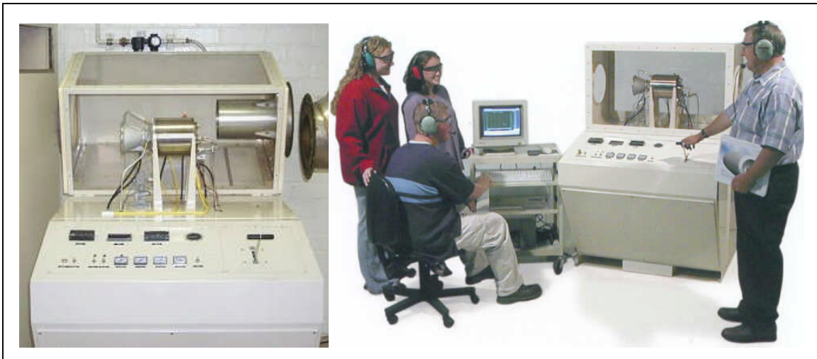
Figure 2. SR-30 front panel and data acquisition system
