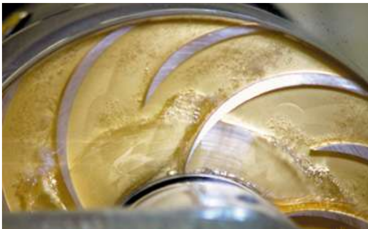
PumpLab's strobe lighting feature allows users to visualize cavitation and other flow phenomena. Source: Turbine Technologies, Inc.
