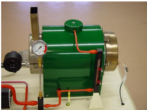
Steam Generation Boiler A dual-pass, flame tube system. If system is cool, open boiler door to reveal boiler construction and flame tube layout. Also note burner fan and tube mounted in door.
