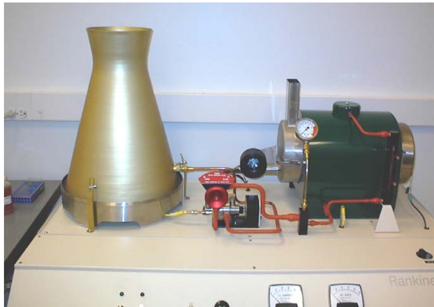
Fig. 1: Photograph of Turbine Technologies' Rankine Cycler .
