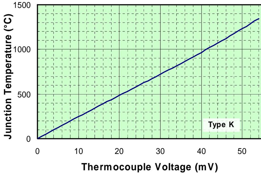
Figure 3. Sensitivity of a standard type-K thermocouple, based on ITS-90 inverse polynomial fit. The millivolt output is based on a reference temperature of 0°C.
