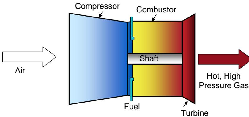
**Figure 9.** Basic components of a gas turbine engine.
