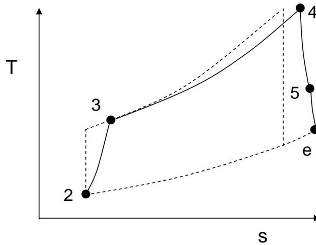
**Figure 13.** Turbojet cycle with nonideal components.
