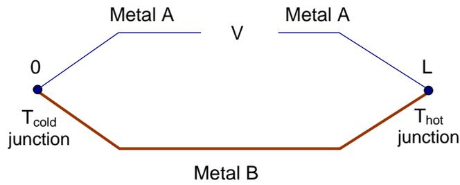
Figure 1. Simple (open) thermoelectric thermocouple circuit.
