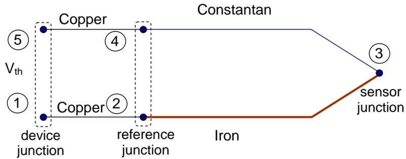
Figure 6. Modified circuit; copper extension wires connect the thermocouple to the measuring device, and the device connections are at the same temperature.
