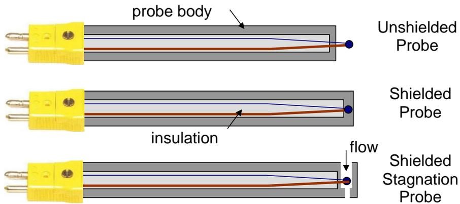
**Figure 8.** Examples of unshielded, shielded and stagnation thermocouple probes.
