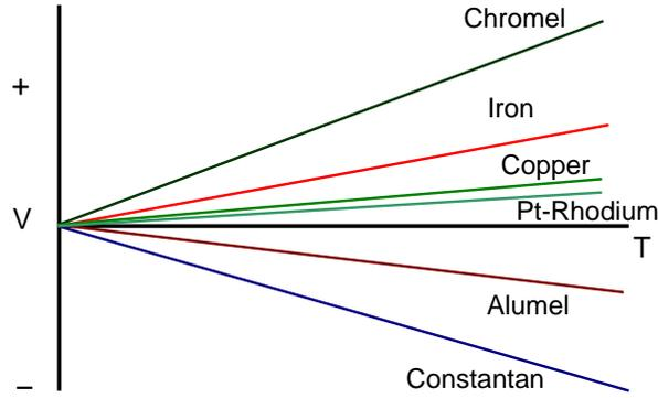
Figure 4. Voltage–temperature response for several metals.
