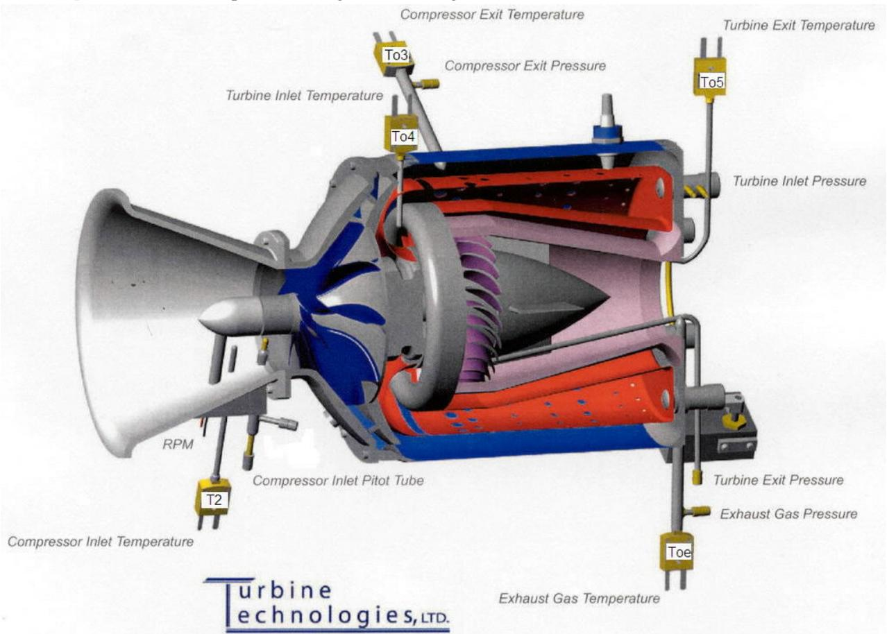
Figure 11. Schematic of the gas turbine system to be used in this lab.
