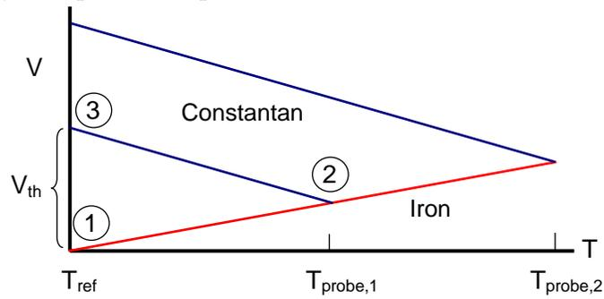
Figure 5. Development of the voltage difference across the thermocouple,  $V_{th}$ , in a thermocouple circuit, like that of Fig. 2, formed by two metals.
