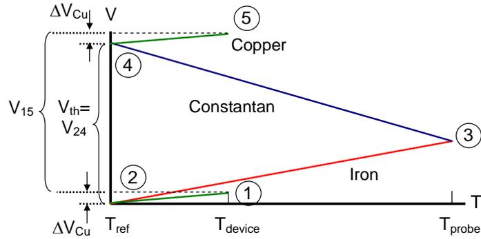
**Figure 7.** Development of the thermocouple voltage difference for the thermocouple circuit shown in Fig. 6. If the wires connecting points 1 to 2, and 4 to 5 are identical, and the temperatures  $T_1$  and  $T_5$  are the same, then the voltage measured across the device ( $V_{15}$ ) is equal to the voltage that would be produced by the ideal thermocouple circuit ( $V_{th}=V_{24}$ ).
