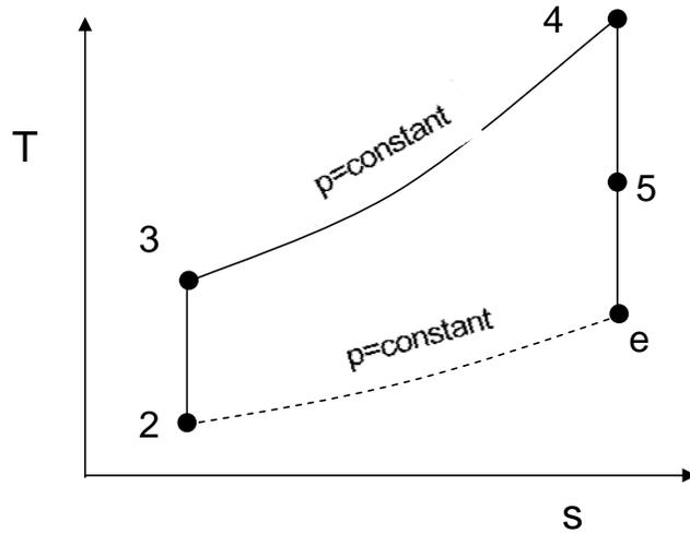
**Figure 12.** Ideal Brayton cycle; stations 2-e correspond to the numbering scheme shown in Fig. 10.
