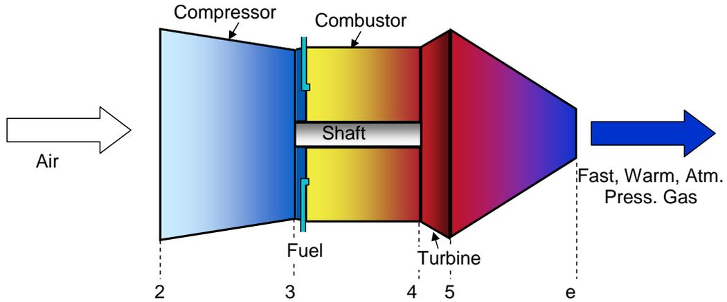
Figure 10. Basic components of a gas turbine engine.
