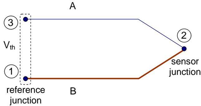
Figure 2. Ideal thermoelectric circuit, with the thermocouple voltage measured across the *isothermal* reference junction.
