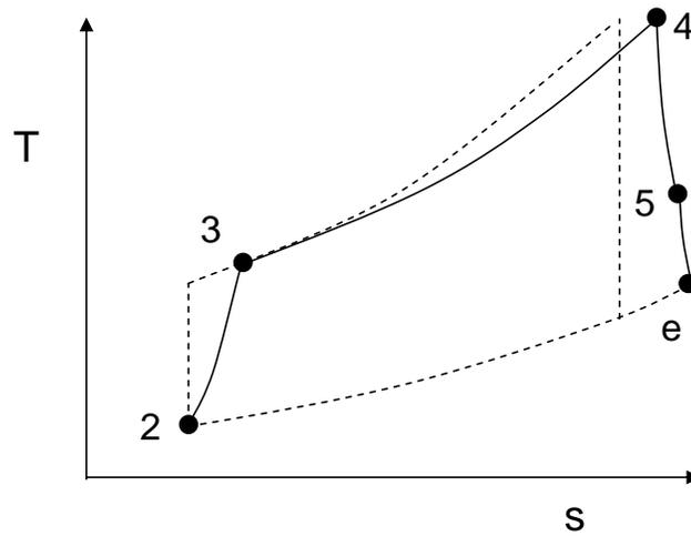
**Figure 13.** Turbojet cycle with nonideal components.
