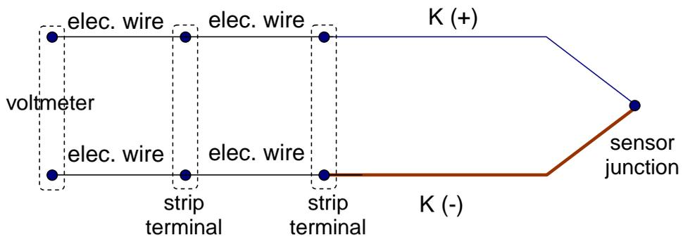
**Figure 14.** Thermocouple circuit to be used in this lab.
