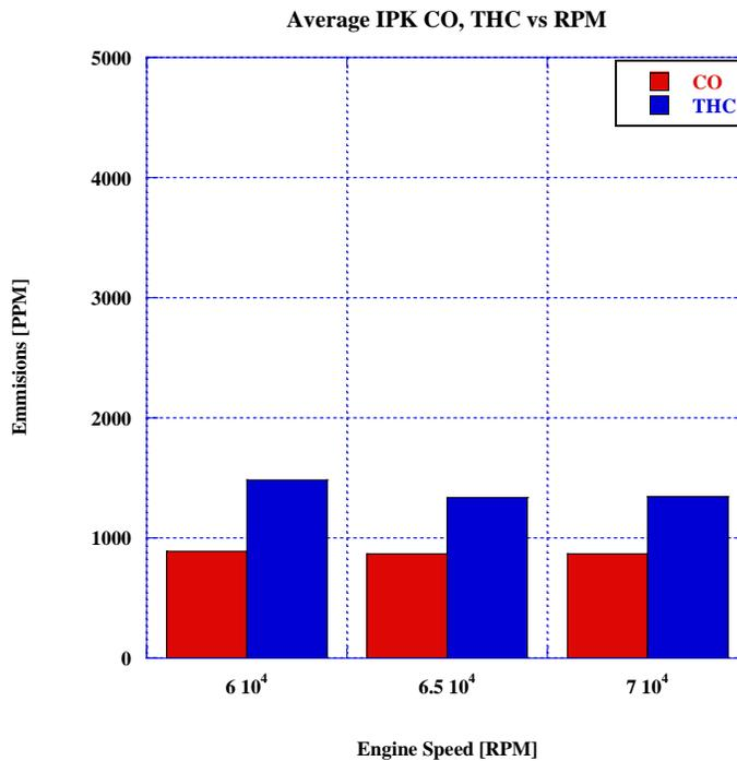
**Figure 23. Average IPK CO, THC Emissions vs RPM**
