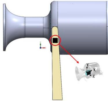
Figure 16. Triaxial Accelerometer Experimental Placement (Kilpatrick 2019)
