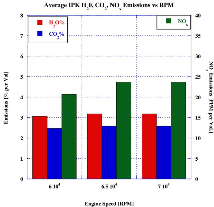
**Figure 21. Average IPK H<sub>2</sub>O, CO<sub>2</sub>, and NO<sub>x</sub> Emissions vs RPM**
