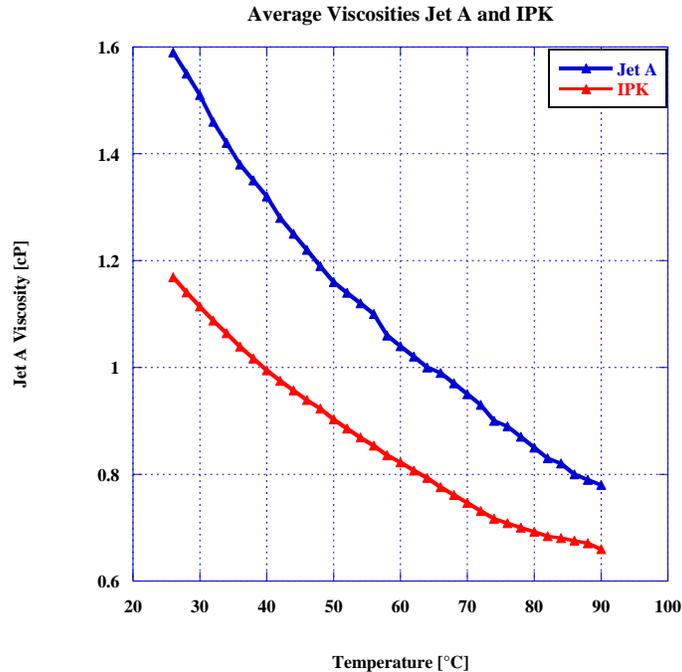
**Figure 5. Dynamic Viscosity of Jet A and IPK**
