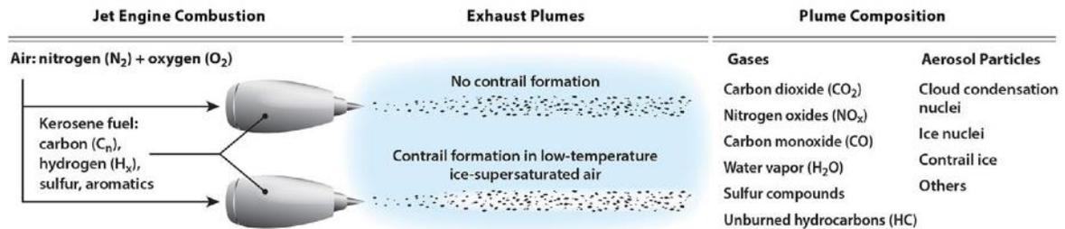
**Figure 1. Emissions from Aircraft at Cruising Altitude (Stein 2020)**
