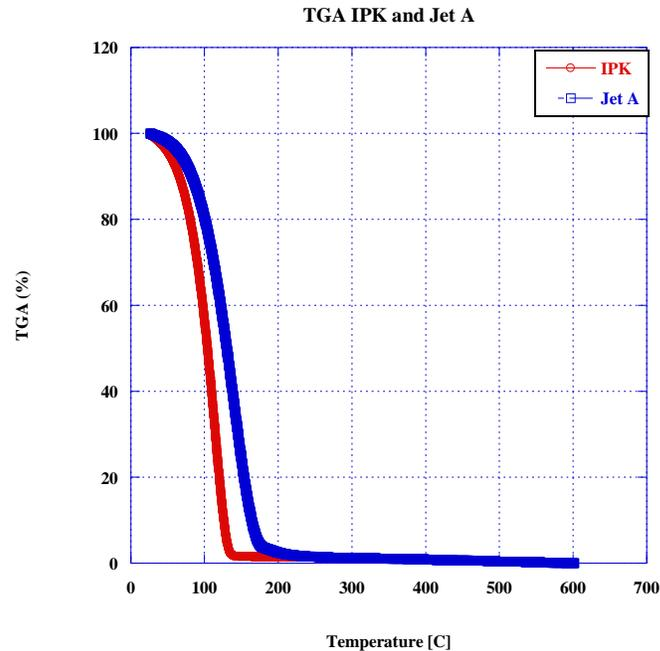
**Figure 6. TGA analysis of IPK and Jet A**
