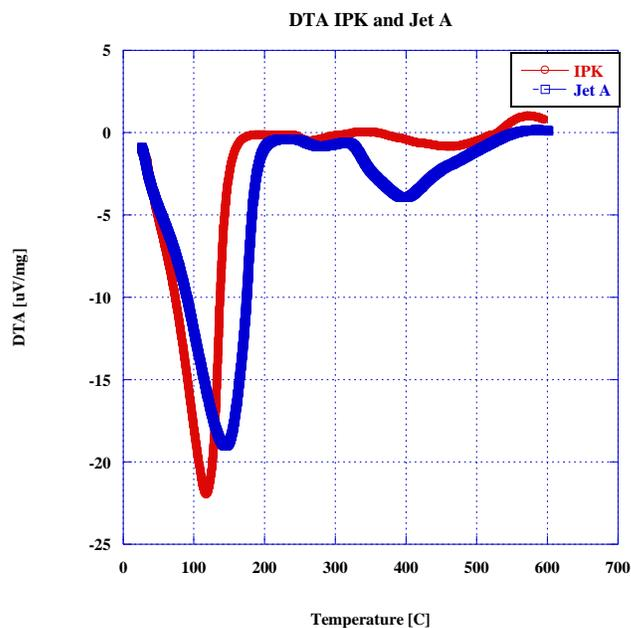
**Figure 7. DTA analysis of IPK and Jet A**
