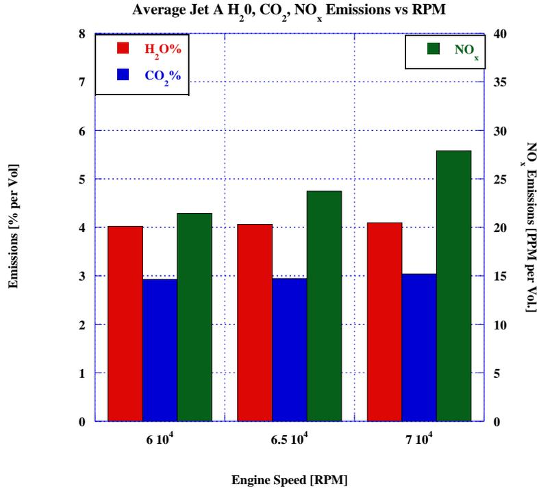
**Figure 20. Average Jet A H<sub>2</sub>O, CO<sub>2</sub>, and NO<sub>x</sub> Emissions vs RPM**
