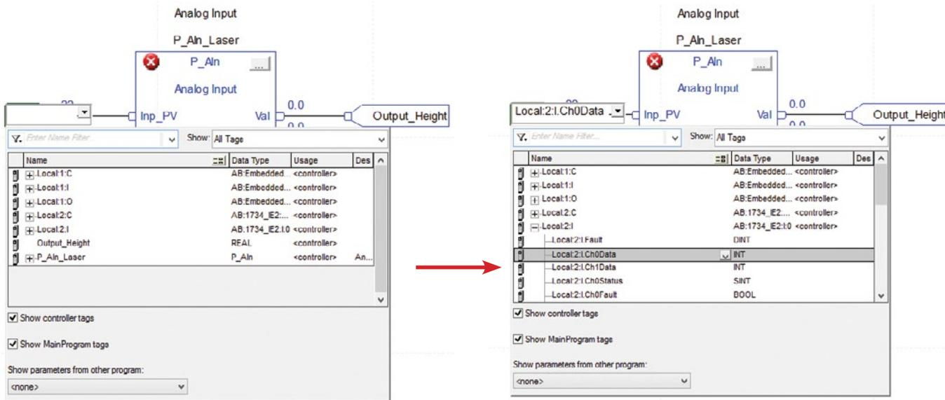
The red X error will go away and the P\_Aln\_Lascr FBD is wired correctly.
