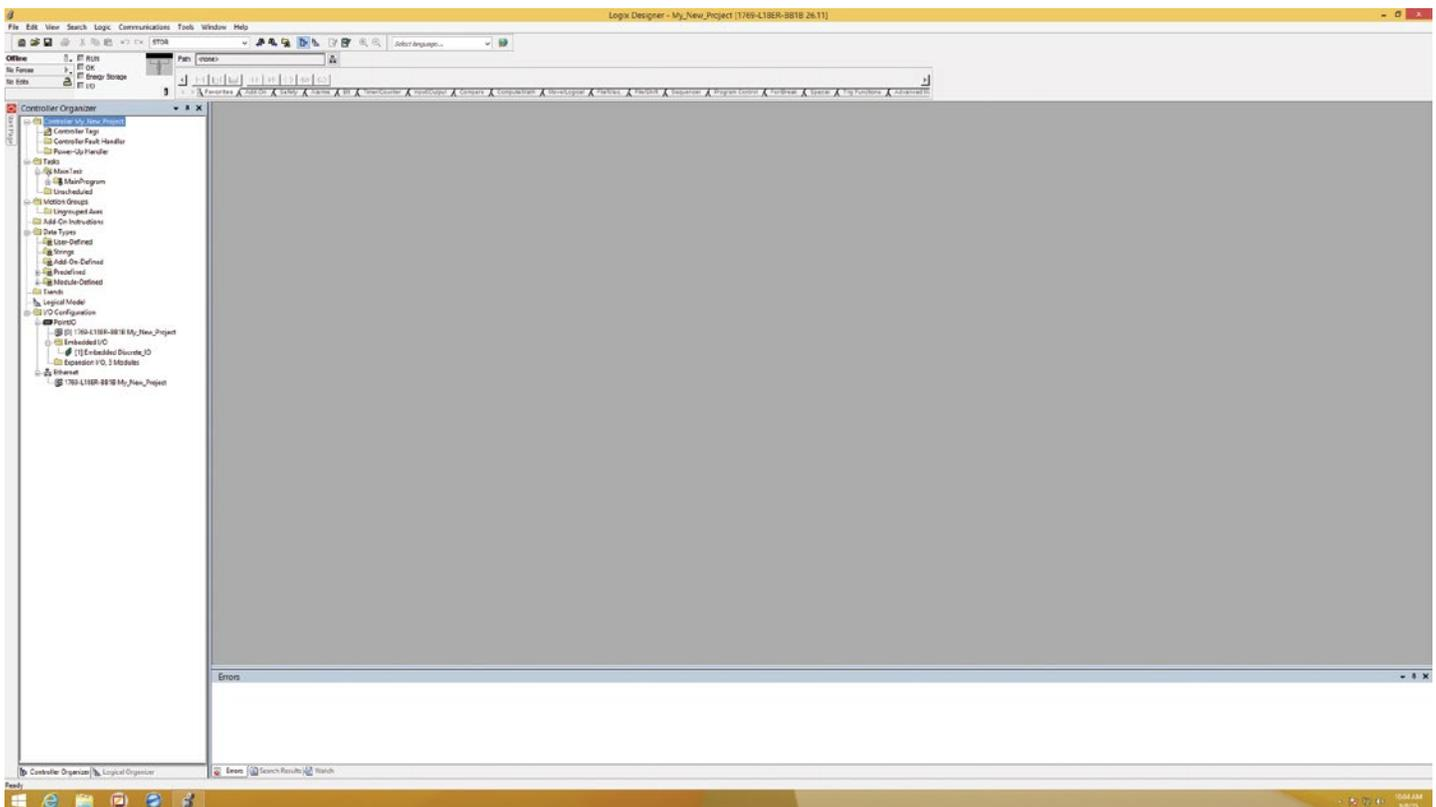
The **Organizer Window** appears on the left side of the Studio 5000 window. There is a folder highlighted for Controller My\_Controls\_Project. There is no I/O, tag database, or logic associated with the controller.
