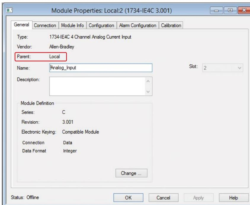
The controller uses different types of connections to transmit I/O data. These connections can be direct connections or rack-optimized connections. *ControlsLab*<sup>TM</sup> uses all direct connections in the communications network. Module connection types are visible in the properties window of the module. See the Parent section for the module. This will determine if the module is local or remote.
