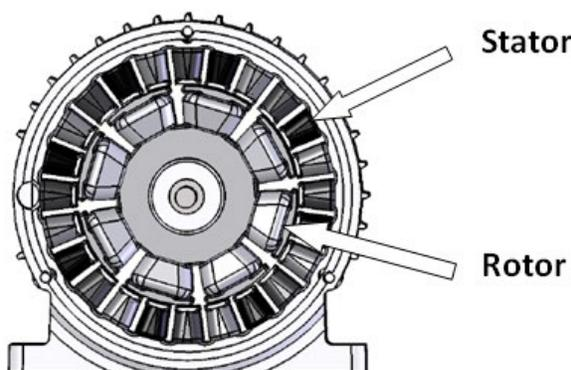
Figure 2.9: Three Phase Motor Cross-Section
