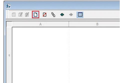
Navigate to the add-on toolbar above the sheet. P\_Motor\_Data should now show up as a button. Click on the button and P\_Motor\_Data AOI will be added to the new function block diagram. The AOI will look like it is empty. We need to enable all of the inputs and outputs that were customized with structured text.
