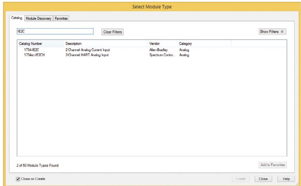
The search is narrowed down to 2 modules of this type. Select the correct module and click **create** to add it to the program.
