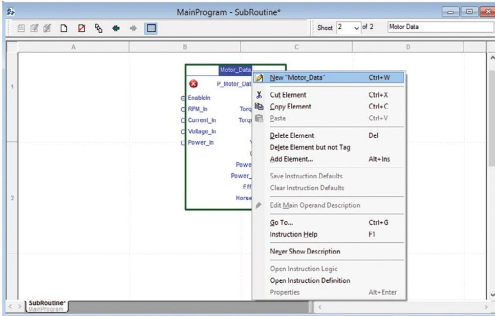
Drag 9 output tags from the tool bar to the function block diagram. Name all of the output tags as shown below. Right-click on each tag and add a new output tag to the scope My\_Controls\_Project. This allows the PAC access to the data calculated from the AOI (since AOI data is local).
