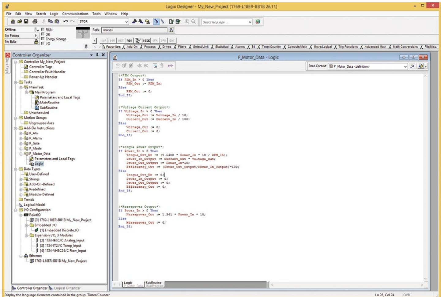
The next step in programming is to wire the P\_Motor\_Data AOI in the function block. Close the logic window for the AOI and open the function block diagram by clicking on the SubRoutine.
