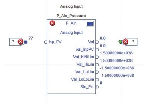
Rename the output tag to Output\_Pressure. Create a new tag in the scope of My\_Controls\_Project and select **Create**. The red X next to Output\_Pressure will go away.
