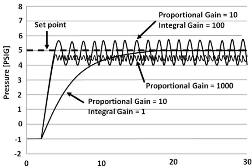
Figure 6.13: Pressure response of the ControlsLab™ to a step change in the pressure setpoint using differing values of the proportional and integral gain.
