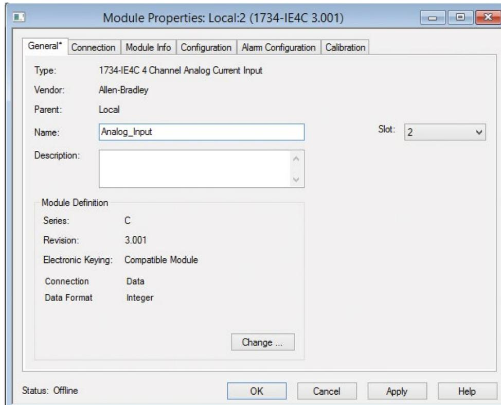
The module configuration should show the module in the correct location with proper naming.
