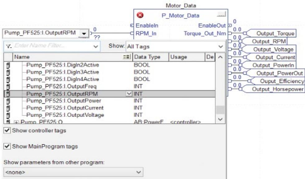
Setup the rest of the VFD tags for P\_Motor\_Data. The finished FBD is shown below. This programming will be used for the Blowing display in FactoryTalk View ME.
