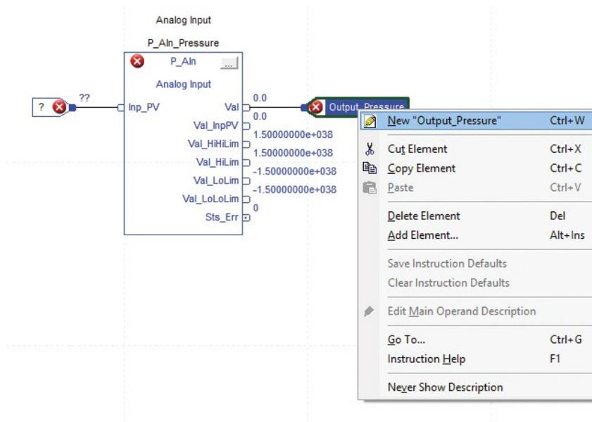
Next we need to wire the input to the proper channel on the 1734-IE2C. Recall that the pressure transducer was connected to.
