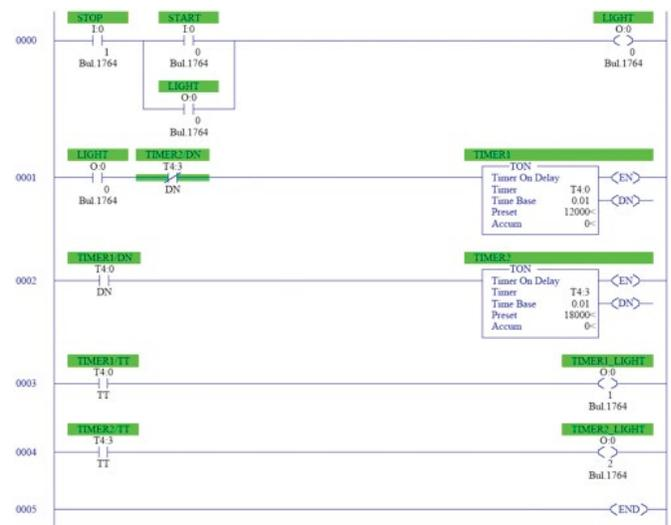
Ladder Logic Rung Diagram
