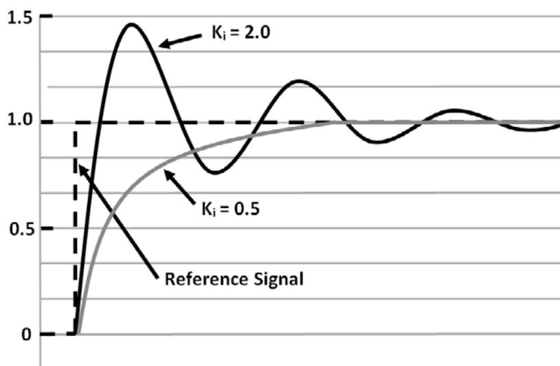
Figure 6.8: Integral responses based on various magnitudes of gain
