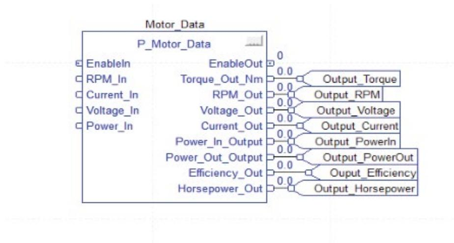
Add four tag inputs to the P\_Motor\_Data function block diagram. Wire the inputs to the 4 input ports.
