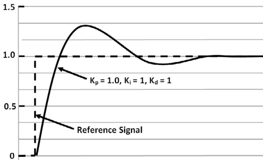
Figure 6.12: A system response using PID Control
