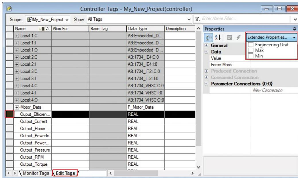
We are going to edit the extended properties of the tag Output\_Efficiency. Select the boxes to add all three properties to the tag. Fields will show up below for the respective boxes. Enter the extended tag data in the boxes. The default values are automatically loaded. Efficiency is a percentage so set the min and max to **0** and **100** respectively. Set the Engineering Unit to **%**.
