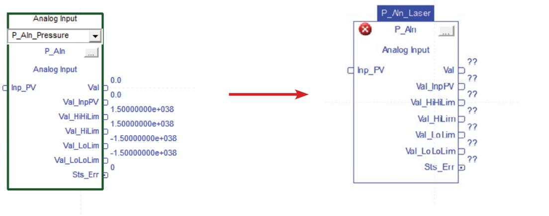
Next, we want to make sure that the tag is stored in the controller. Right-click on the tag and select **New "P\_Aln\_Pressure"**
