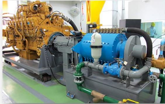
*Figure 2-1: Industrial Diesel Dynamometer*
