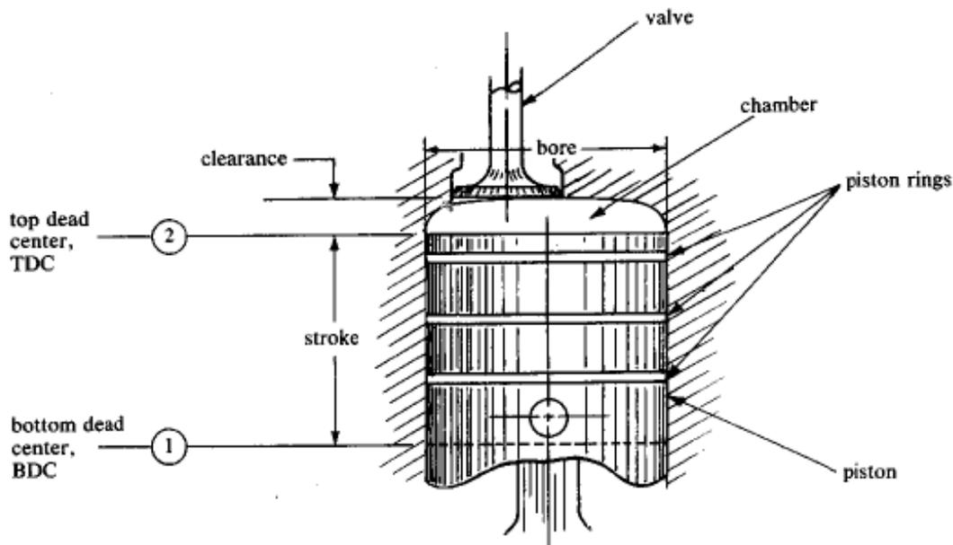
Figure 1-8: Common IC engine parameters
