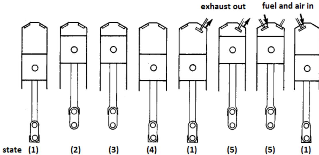
Figure 1-5: Four-stroke Otto Cycle
