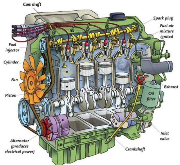
Figure 1-1: Internal Combustion Engine Cut-Away
