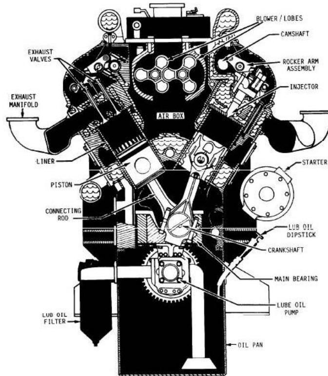
*Figure 1-12: Cross-sectional view of typical V Configuration two-stroke-cycle diesel engine*
