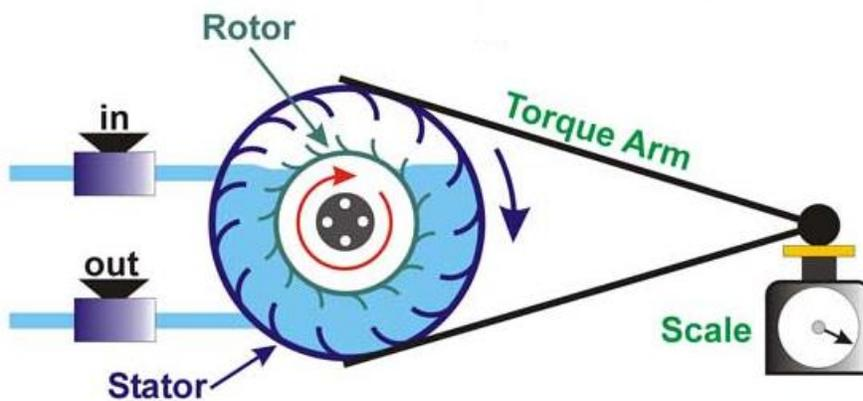
Figure 2-4: Water Brake Dynamometer Schematic
