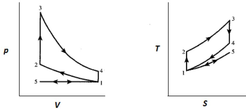
Figure 1-6: Property diagrams for the four-stroke Otto cycle
