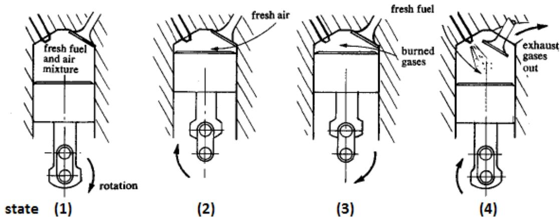
*Figure 1-11: Physical Operations of the Diesel Engine*
