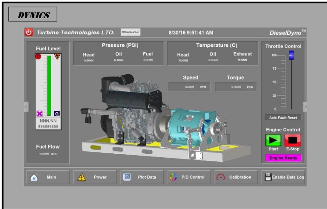
Dynics™ Human Machine Interface (HMI) with Allen Bradley Studio 5000™ and FactoryTalk™ Automation Programming Software Loaded
