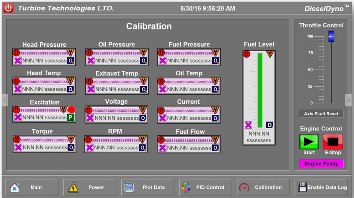
HMI Sensor Calibration Screen
