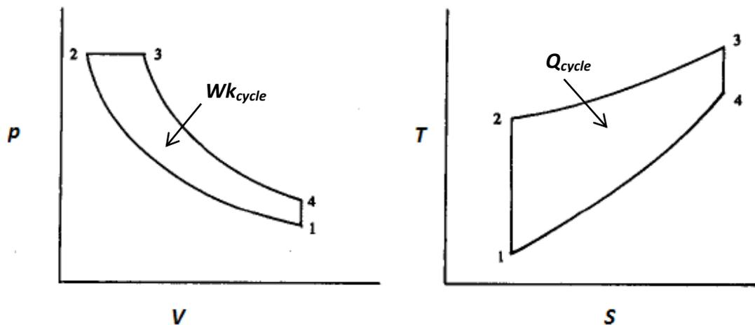
Figure 1-10: Property diagrams for ideal diesel cycle
