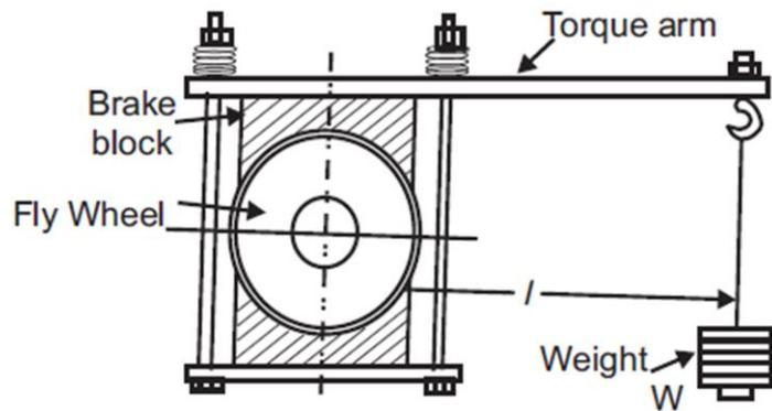
Figure 2-2: Prony Brake (Rope with balance springs)    Figure 2-3: Prony Brake (Torque Arm)
