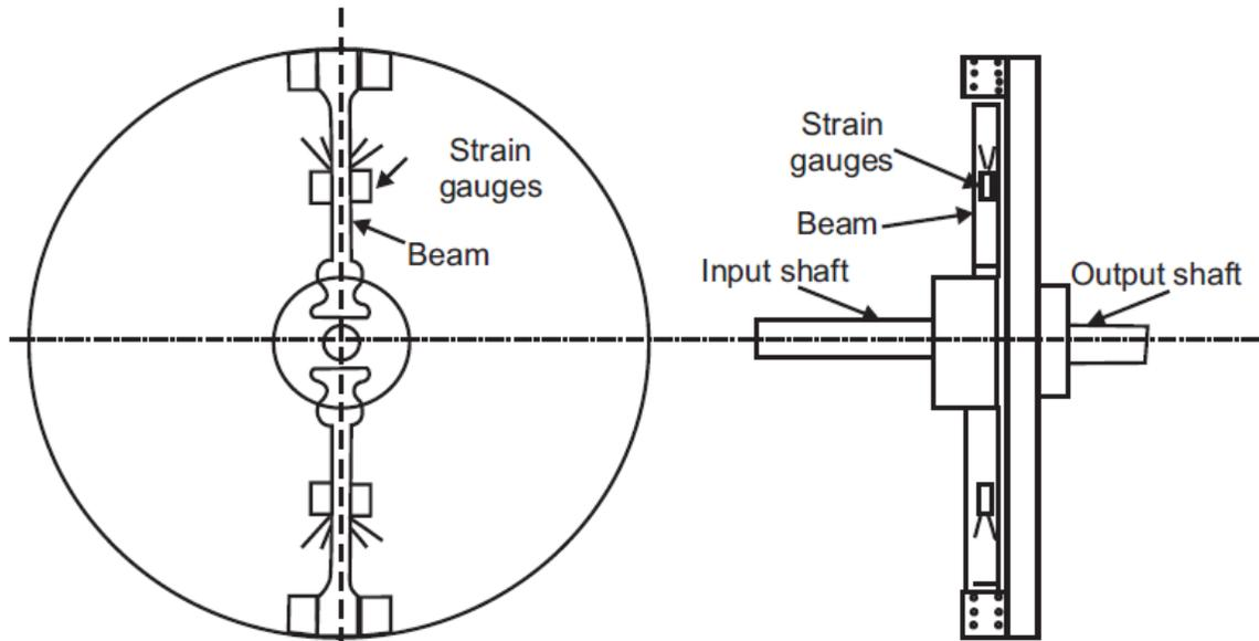
*Figure 2-6: Transmission Dynamometer*
