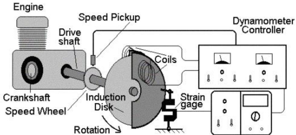
Figure 2-5: Eddy-Current Brake Dynamometer Schematic
