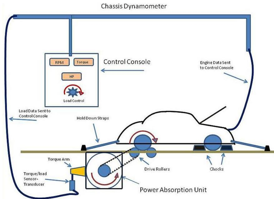
*Figure 2-7: Chassis Dynamometer Configuration*
