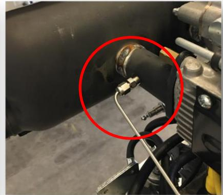
Engine Exhaust Gas Temperature
