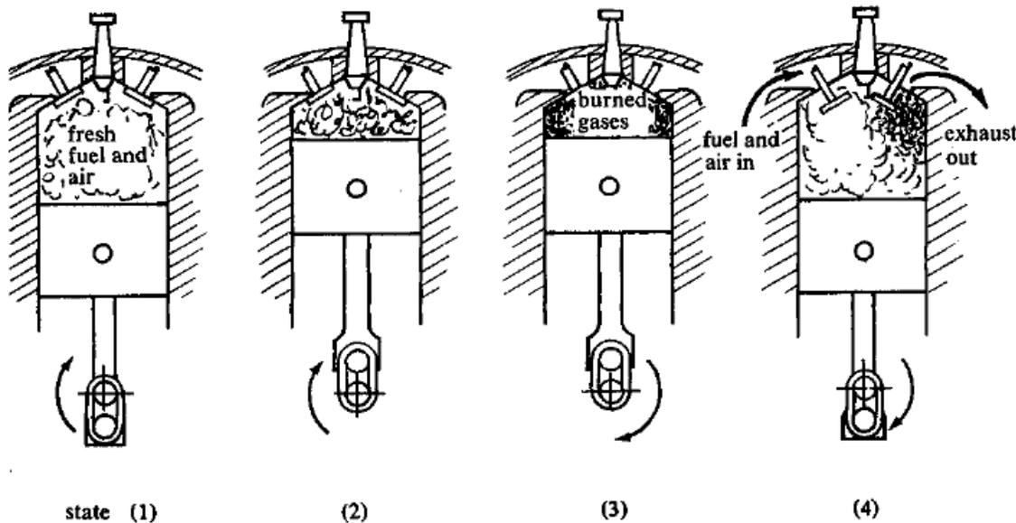
Figure 1-4: The Otto Cycle application in a piston-cylinder device
