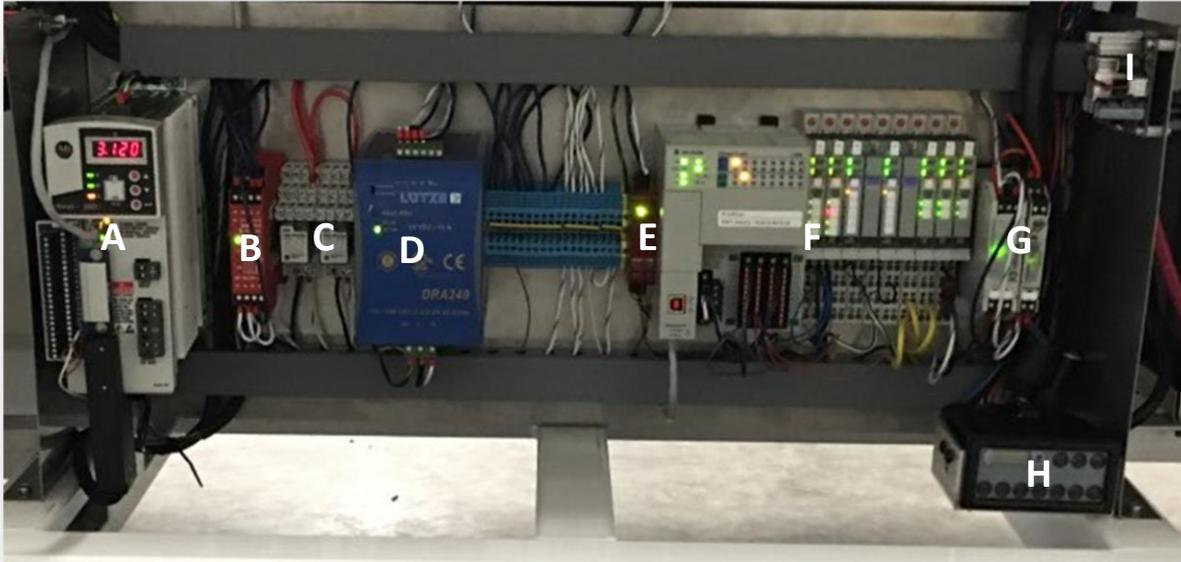
A: Engine Throttle Servo Drive
