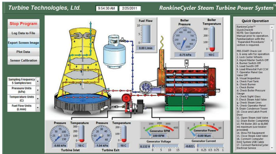
Figure 2.12: Virtual Instrument Panel
