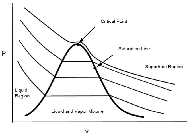
Figure 1.12: P-v diagram of steam-water phase change
