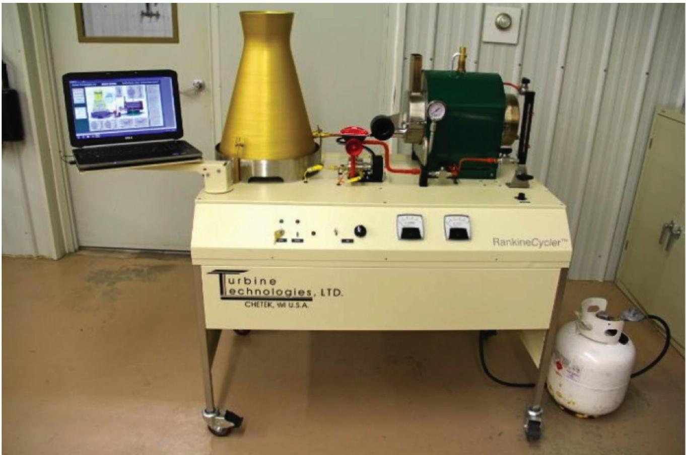
Figure 2.1: RankineCycler™ System Features
