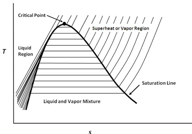
Figure 1.11: T-s diagram of steam-water phase change
