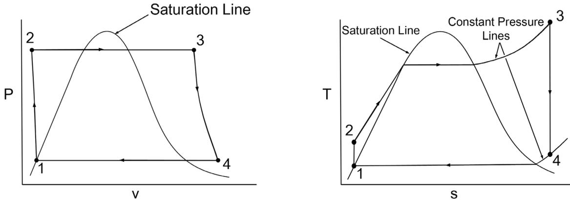
Figure 1.14: Property Diagrams of the Rankine Cycle
