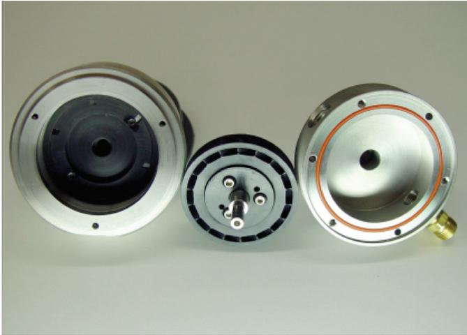
Figure 2.7: Impulse Steam Turbine Wheel
