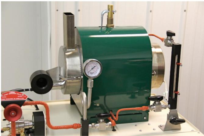
Figure 2.3: ASME Flame Tube Water Boiler
