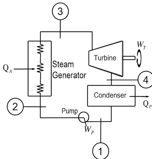
Figure 1.13: Typical schematic of the Rankine Cycle
