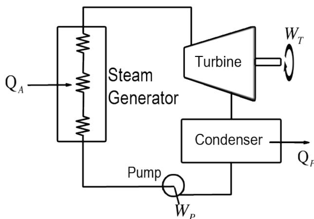
*Figure 1.10: Typical schematic of the Rankine Cycle*
