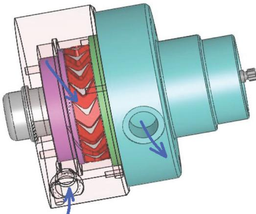
Figure 2.8: Steam Turbine CAD Cutaway
