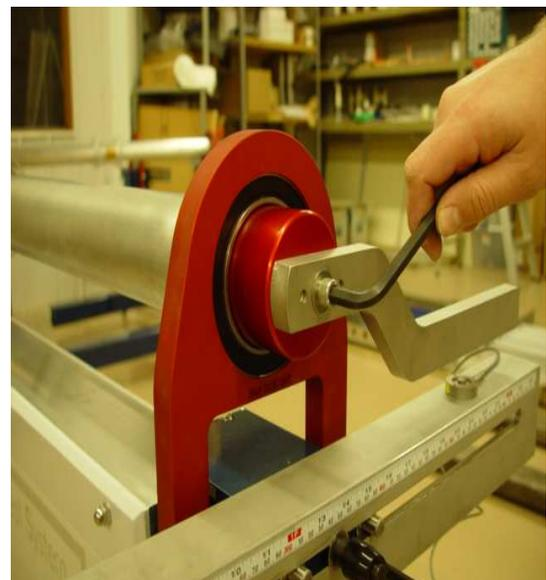
*Tighten Torque Arm Bolt securely with Allen Wrench.*
