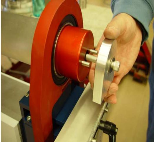
*Insert Cantilever Load Block on red end.*
