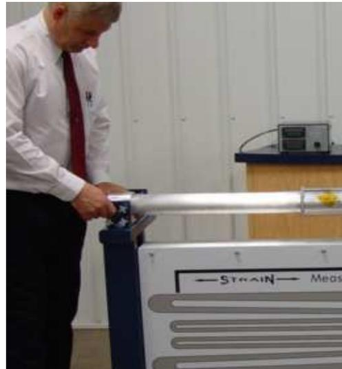
*Tighten block end knobs fully. Then tighten red yoke knobs securely.*
