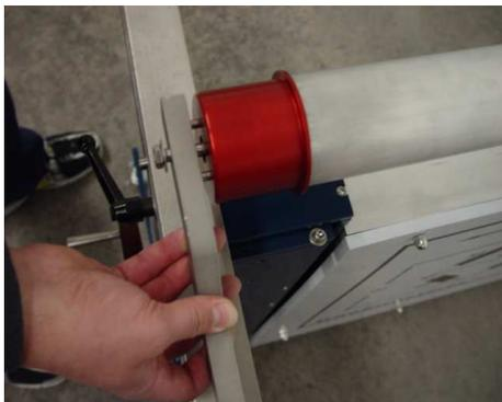
Insert Torque Arm into Tube End.
