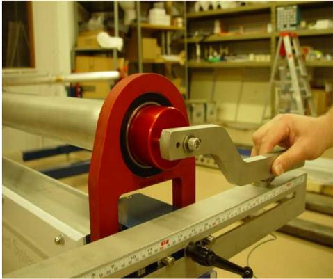
Loosen Torque Arm with Allen Wrench and remove.
