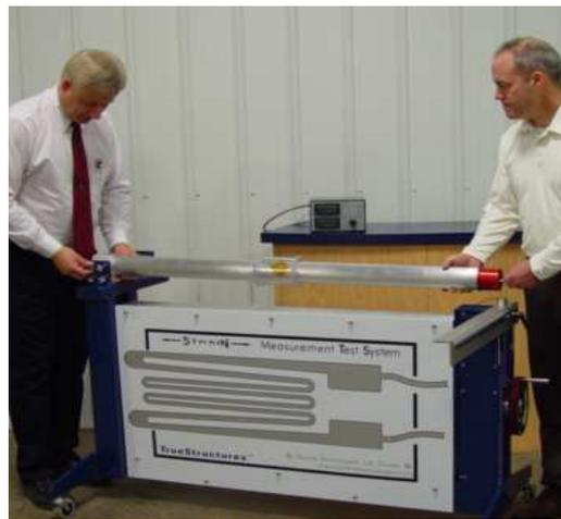
Position tube in cantilever position, tighten hand knobs while pulling up on tube end..
