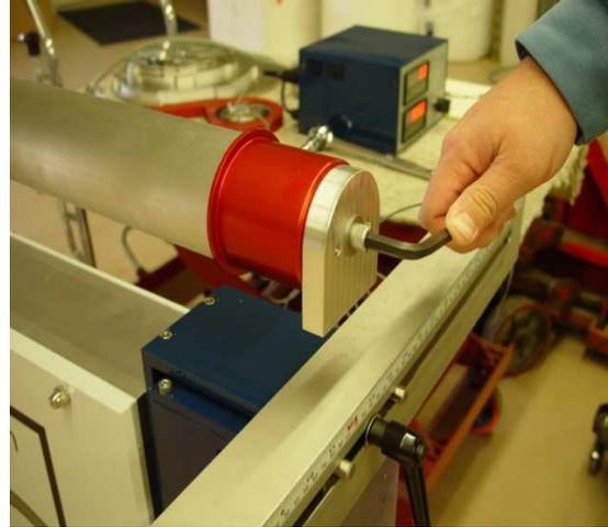
*Tighten Load Block with Allen Wrench.*
