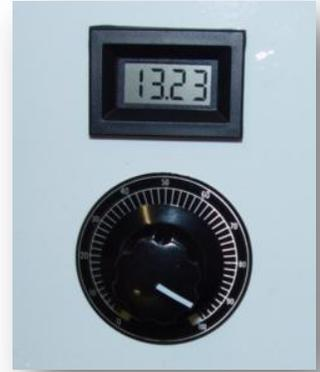
6. Adjust each **PHASE LOAD** rheostat (A, B, C) from 0 Ohms to 10 Ohms and let system stabilize (10 seconds). This is considered balanced loading. Again, performance data will be recorded by the data acquisition system. Make sure you record these settings as the Data Acquisition system does not record it.
